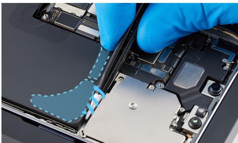
11. Repeat steps 9 and 10 to remove the remaining battery adhesive strip from the top of the battery. If you remove the entire strip, continue to step 12.
