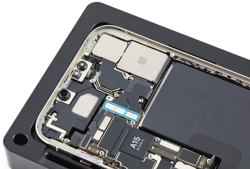
6. Gently hold the camera flex cables together (1) and lift the cameras out of the enclosure (2).
