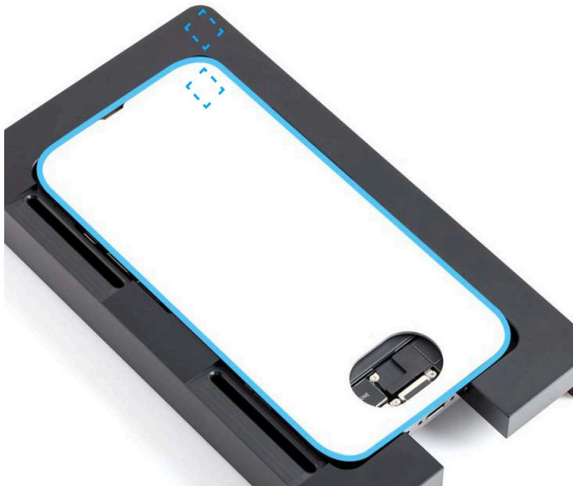
8. Position the repair tray with the iPhone in the display press. Pull down the lever until the display press locks.
