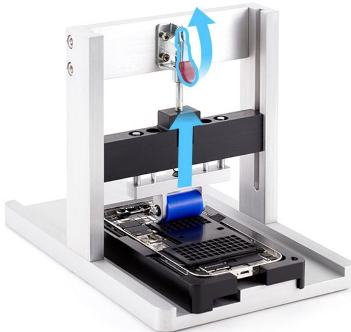
14. Remove the repair tray from the battery press.
