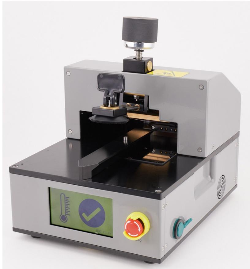
3. Take the iPhone out of the repair tray. Then insert the iPhone into the heated display pocket with the display faceup and the Lightning connector facing the bottom of the pocket.
