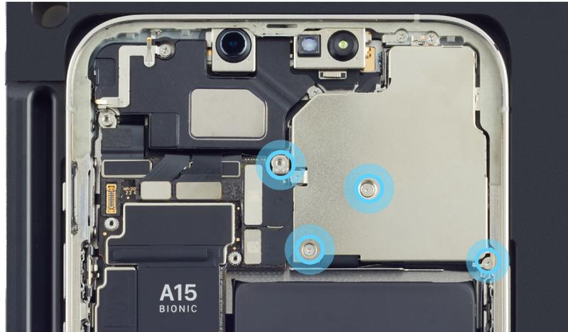
3. Use a torque driver and the JCIS bit to remove the crosshead screw from the camera cowling. Set aside the screw.
