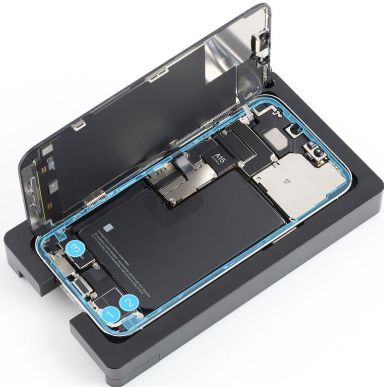
22. Inspect the display adhesive to ensure that it's in the correct position and not damaged or wrinkled. If the adhesive is damaged, remove it and apply replacement adhesive.
