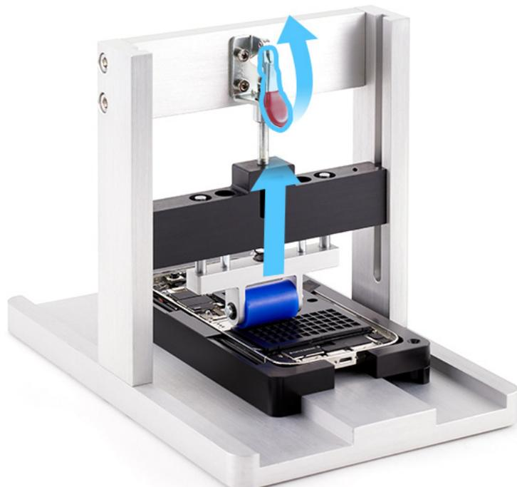
10. Position the repair tray and enclosure onto the battery press with the right slot over the pin.
