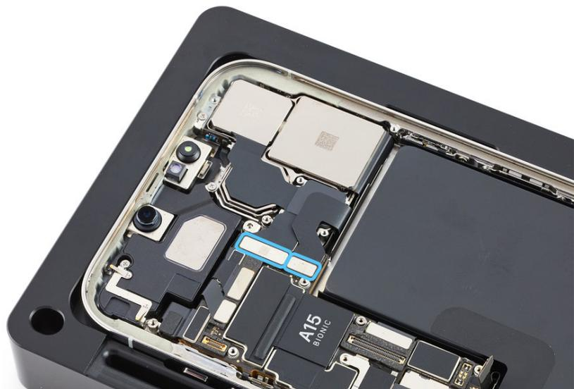
5. Lightly press the cameras into the enclosure.
