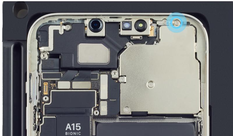
4. Use ESD-safe tweezers to tilt up the camera cawling from the left side (1). Then slide the cawling tabs out of the slots on the right side of the enclosure (2). Save the cawling for reassembly.
