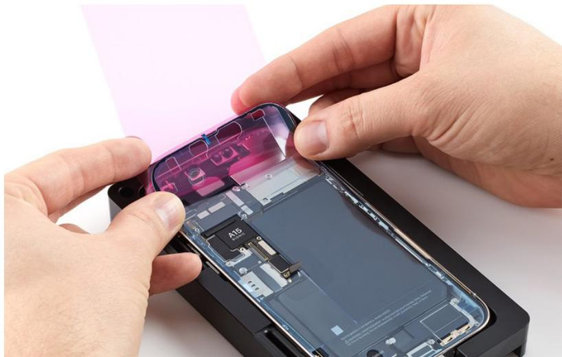
6. Use the flat end of the black stick to gently adhere the grounding foam as shown.
