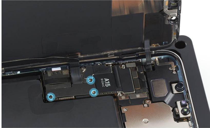
18. Use ESD-safe tweezers to slide the tab of the upper cawling behind the ambient light sensor flex cable. Then lower the cawling over the end of the flex cable.
