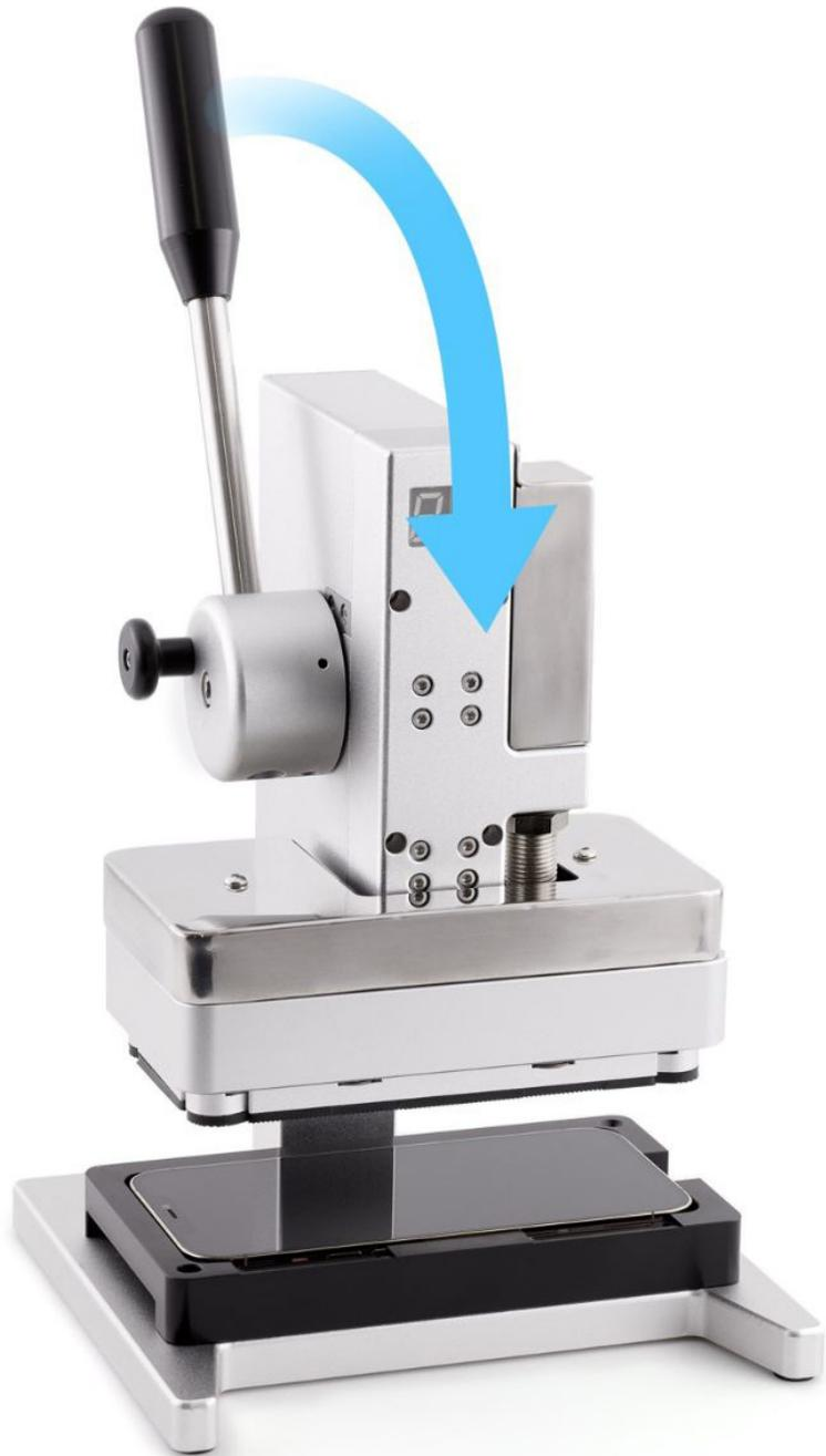
28. Wait until the timer on the display press beeps. Pull down the lever (1) and pull out the release knob (2). Then lift the lever (3).
