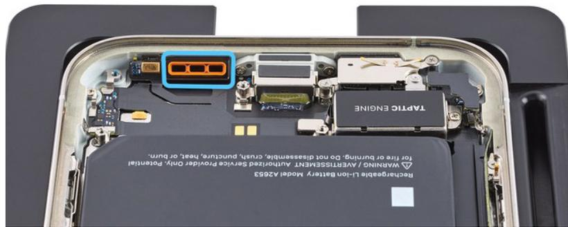
2. Rotate the repair tray. Then position the bottom speaker in the enclosure.
