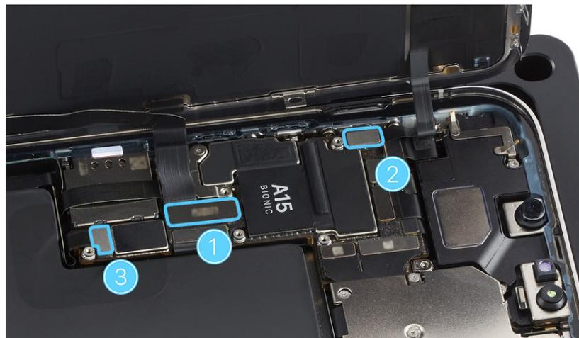
16. Use ESD-safe tweezers to position the lower cawling over the ends of the display and battery flex cables.
