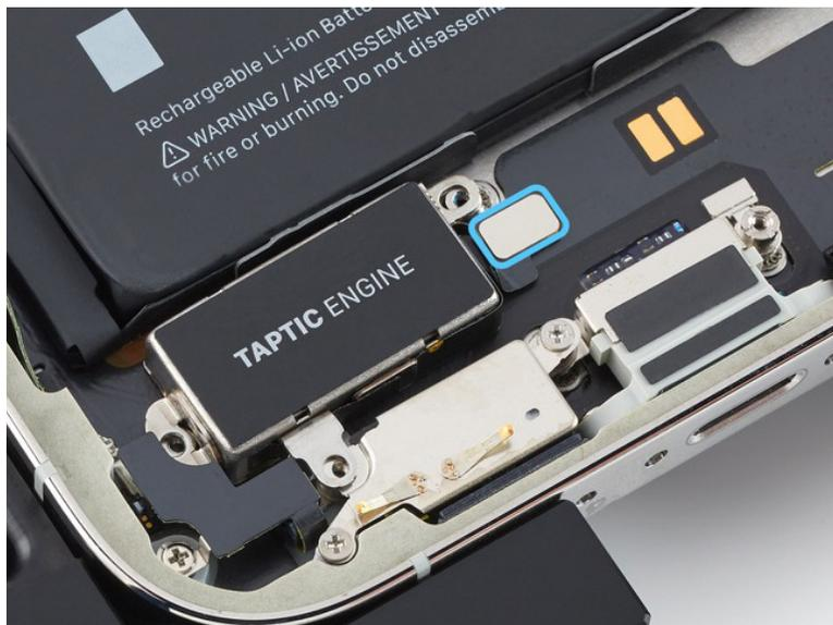
4. Use the blue torque driver and super screw bit to install one new super screw into the Taptic Engine (1).
