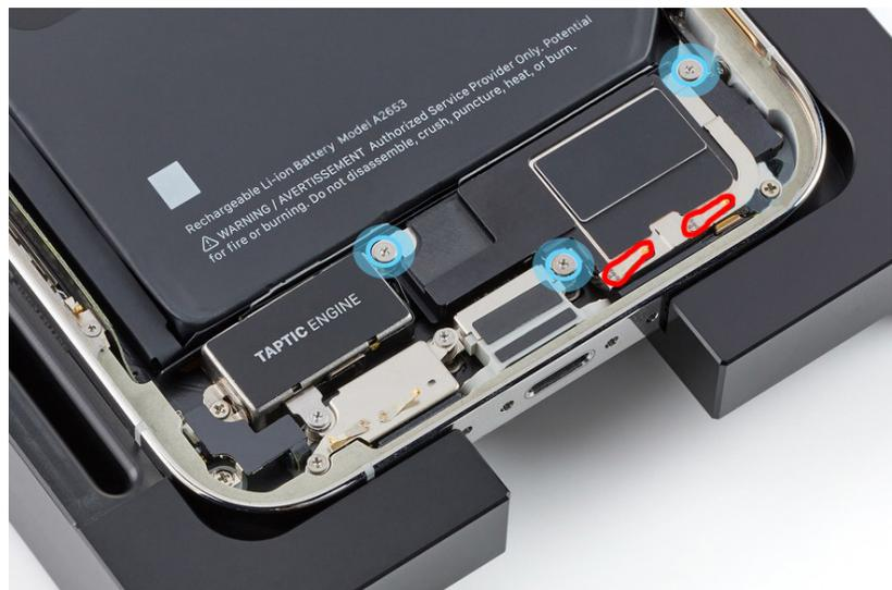
4. Use the blue torque driver and JCIS bit to install one new crosshead screw into the bottom speaker.
