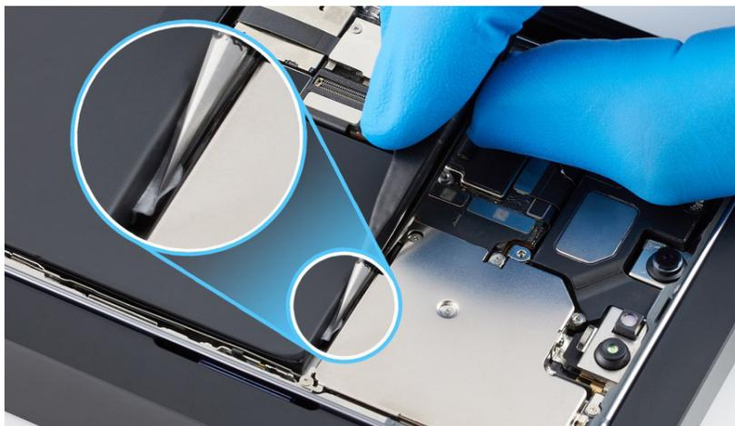
10. Keep the tweezers in the channel between the battery and the camera cowling. Continue to slowly twist the tweezers until you've removed the entire adhesive strip.
