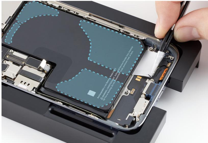
6. Use ESD-safe tweezers to grasp the bottom left battery adhesive tab. Gently peel the adhesive tab away from the battery.
