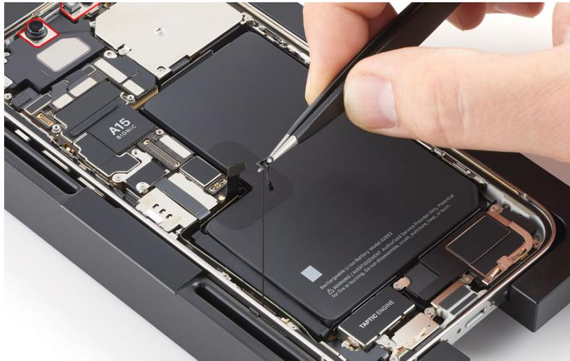
30. Use ESD-safe tweezers to remove the grounding foam from the top of the enclosure above the TrueDepth camera.
