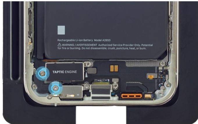
4. Lift the end of the Taptic Engine flex cable off the connector.
