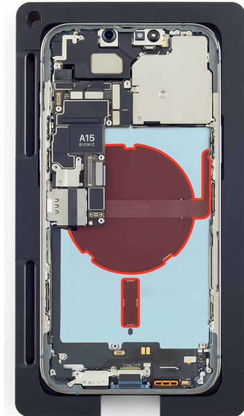
2. Reinstall the [Taptic Engine](#).
